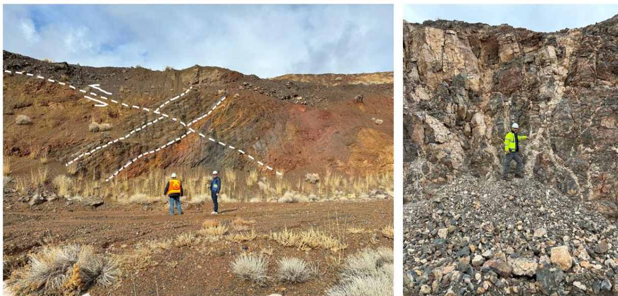
Figure 12-60: GRE's QP Geological Inspections in 2024, Fault and Q-Veins in Grass Valley Formation
